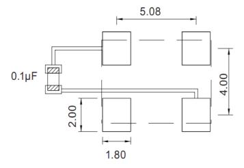
To ensure optimal oscillator performance, place a by-pass capacitor of 0.1uF as close to the part as possible between Vdd and GND pads.
