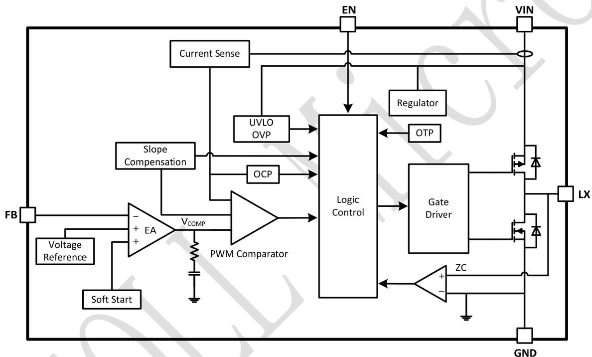
Figure 2. TMI3108 Block Diagram
