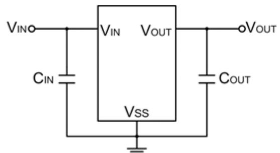
For CJ75XXS series, input and output capacitors are required to achieve stability and help the equipment obtain better transient response and PSRR. It is recommended to use 1 $\mu$ F input and 1 $\mu$ F output capacitors.
